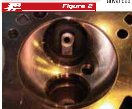
**Figures 1 & 2:** The location of the spark plug has an effect on ignition timing. The head design normally dictates where the plug can be located. By having the plug closer to the center of the bore it allows the timing advance to be reduced or retarded because the burn rate is increased. Notice how the head on the right allows the spark plug to be located closer to the center, the head on the left must be offset more.
