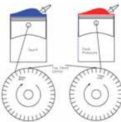
The picture on the left illustrates the crank position at the point of spark ignition. The picture on the right shows the general location where peak pressure inside the cylinder should occur. This helps illustrate how retarding or advancing the ignition timing can change the point where peak pressure occurs in the cylinder.
