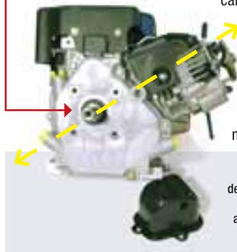
can also be done by sticking a pencil in the spark plug hole and slowly turning the engine over until the engine reaches its highest position.
