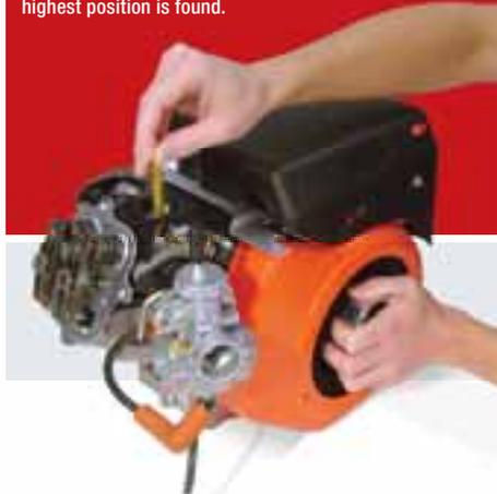
by hand. What this does is slightly lift the valve on the compression stroke to relieve some of the pressure so it can be turned over easily. This release then swings out of the way when the engine reaches operating speed. The lash can't be set on this compression release or the setting will be dramatically wrong. By setting the lash a little past TDC you eliminate the possibility of running into this.
