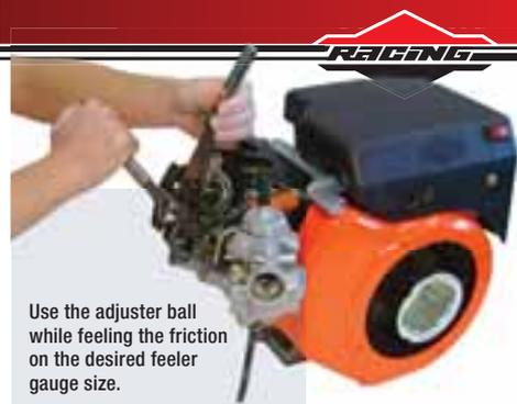
Use the adjuster ball while feeling the friction on the desired feeler gauge size.
