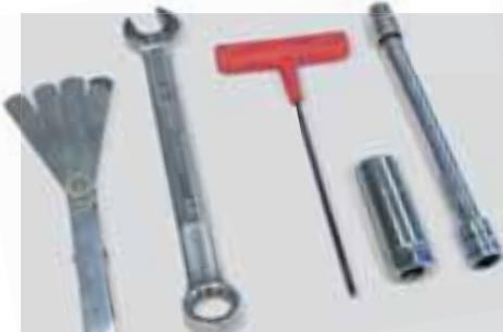
Only a couple of common tools are needed to set the lash on the Animal. A 5/8" std wrench, 1/8" Allen wrench, 10mm and/or 3/8" socket, spark plug socket, and feeler gauges.
