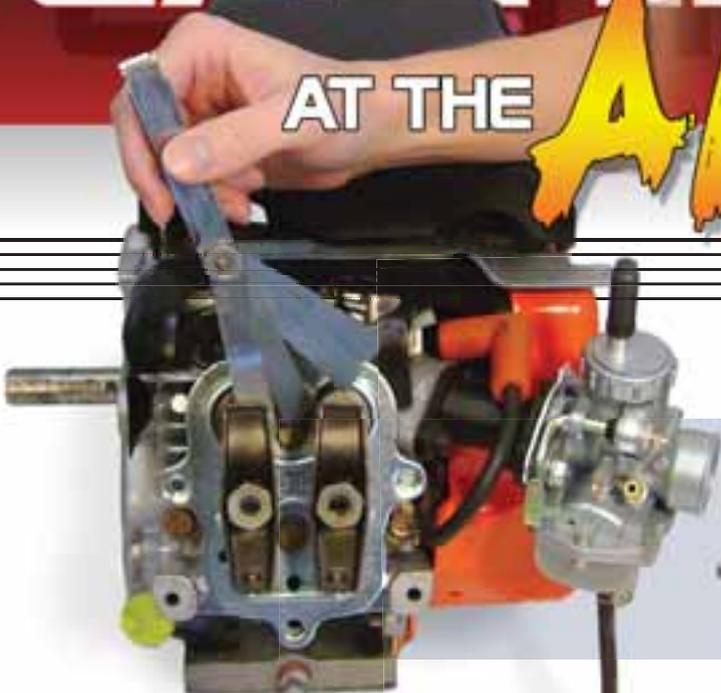
apart, and the second comes from wear of the related components. If the engine is taken apart or has had the head, rocker arms, or side cover removed in the tech barn, a valve lash check and possible adjustment are warranted. The main
