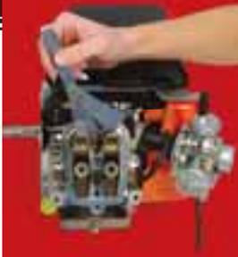
The feeler gauge is inserted between the rocker arm and the valve. Different feeler gauges should be tried until a little friction is felt but it cannot be sticky or loose, the size of this gauge is then your lash.
