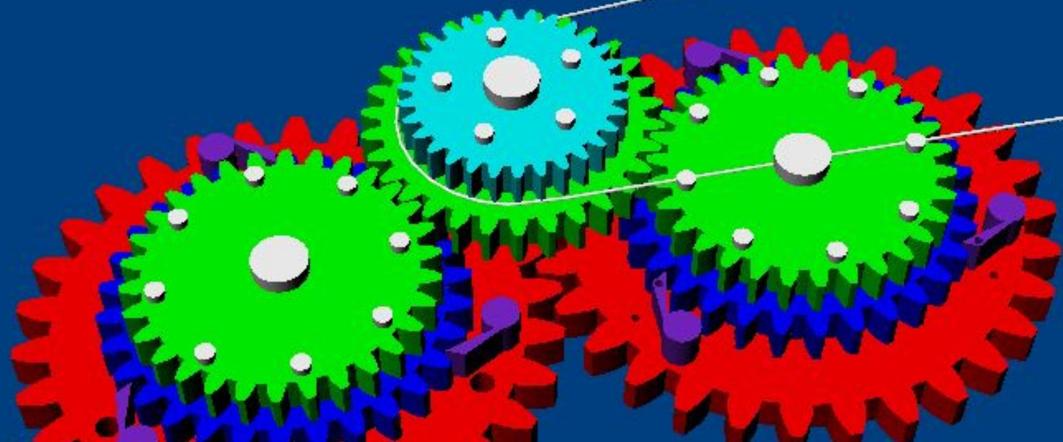
**Both click-wheels are identical except the front (closest to the peddles) click-wheel has three peg holes to keep the paws **ENGAGED** when rotating in either direction. The rear click-wheel has three peg holes to keep the paws **DISENGAGED** when rotating in either direction. These holes are for pegs to be inserted when changing modes. With no pegs inserted, this is mode three, the bi-directional mode.**
