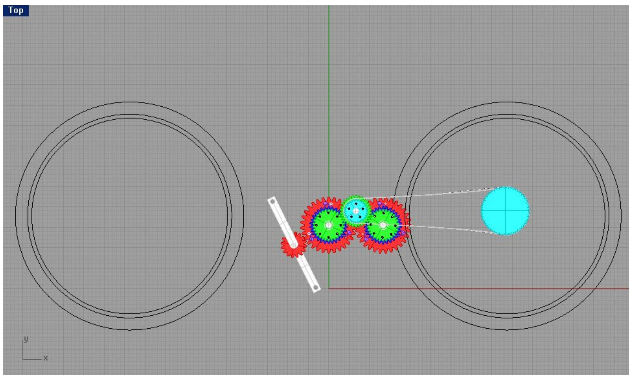
**Each click-wheel consists of three gears. Eight bolts fix the top two gears to each other. The bottom gear retains the top gear assembly, but still allows it to rotate. The bottom gear also has three spring loaded ratchet paws. These ratchet paws only turn the top gear assembly in one direction. If the bottom gear is turned in a counter-clockwise direction, the paws will just slip past the top gear assembly, not turning it.**
