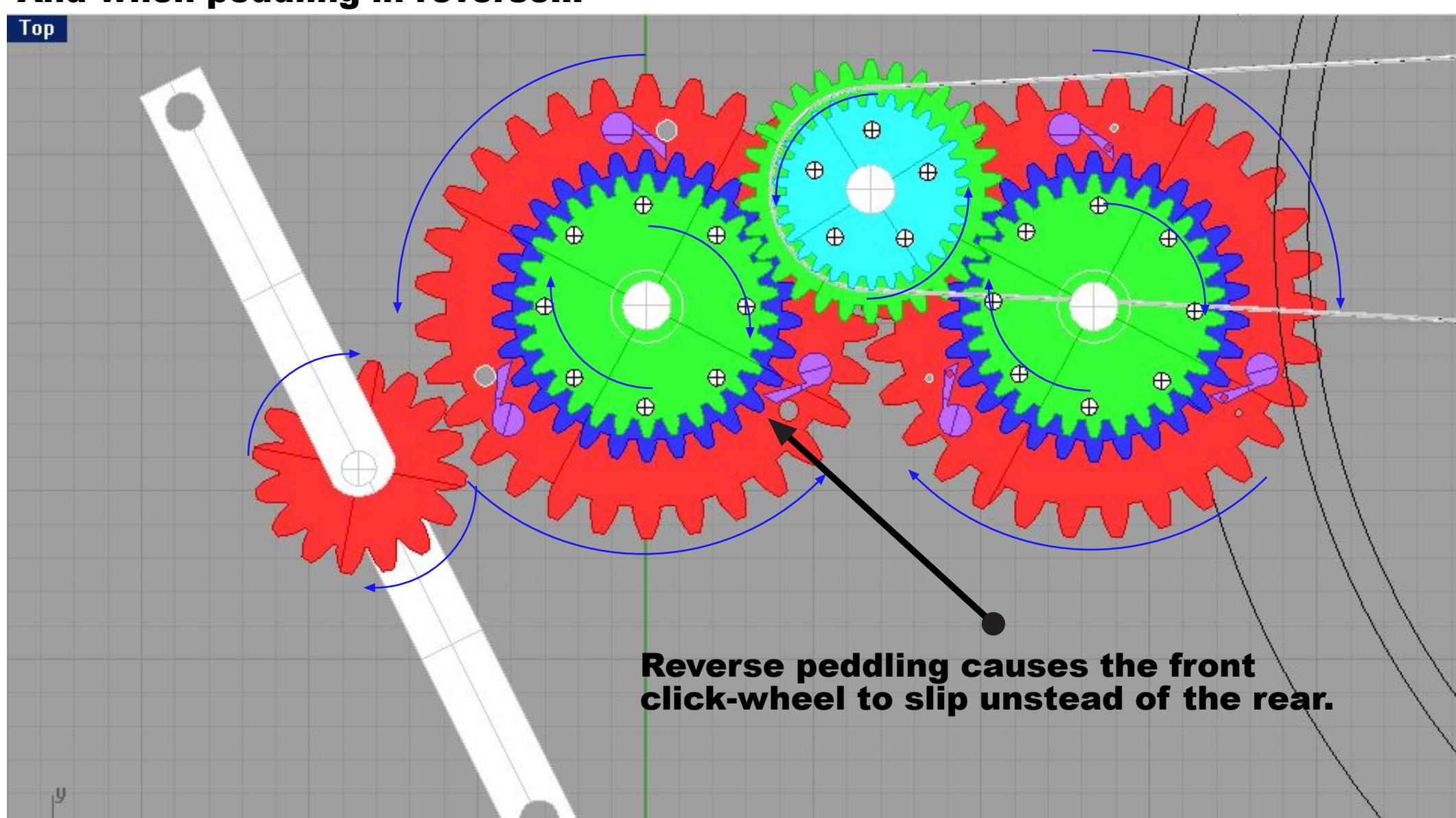
**The second mode, a regular bicycle. We place the pegs in the rear click-wheel. This prevents the ratchet paws from ever coming in contact with the upper gear assembly. This means peddling backwards will have no effect. Now the front click-wheel acts like a rear one-way hub would.**
