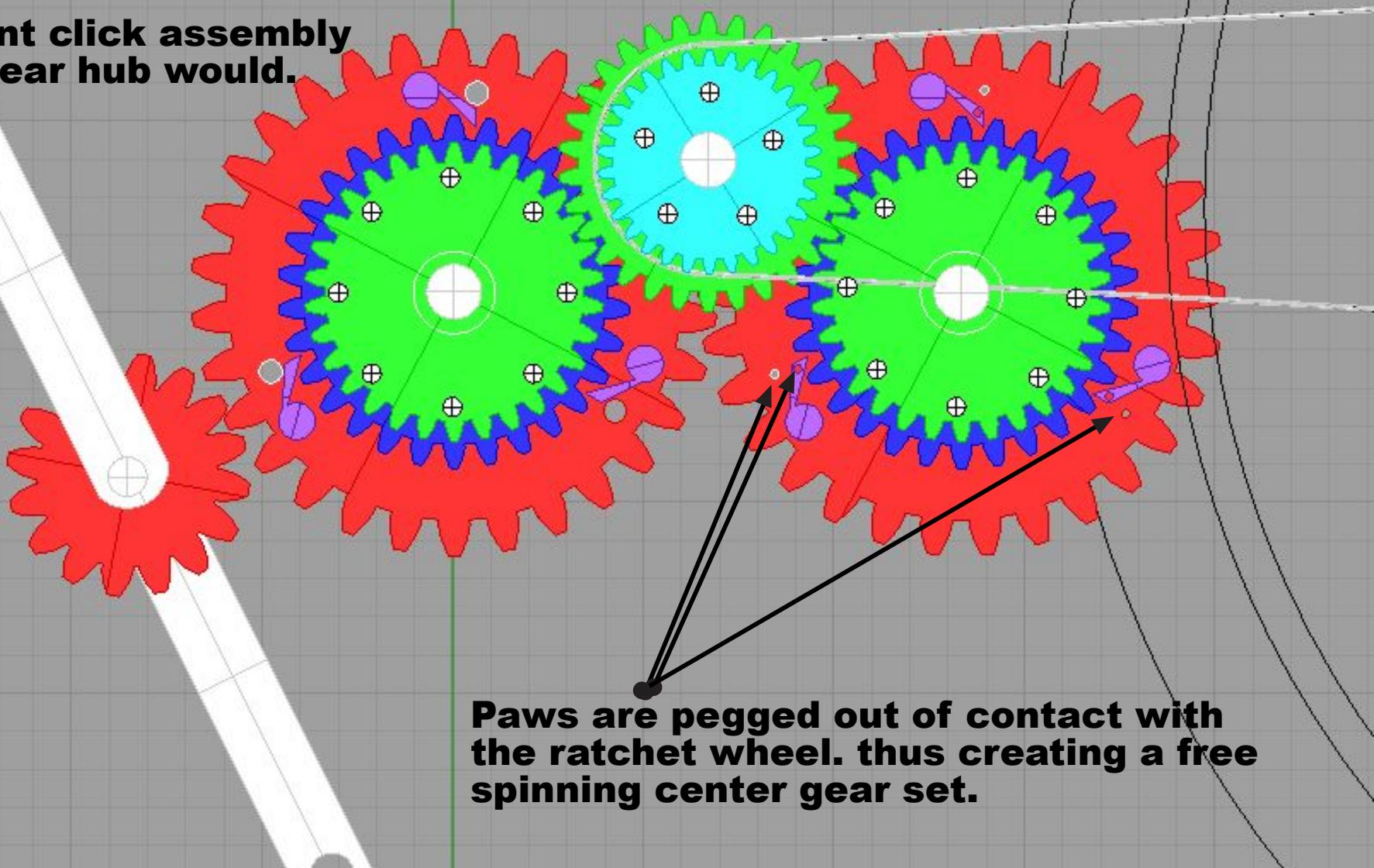
**Finely, the fixed gear mode. Pegs are to be installed in the rear click-wheel as before, so the rear click-wheel has no effect on the mechanism. Also the front click-wheel will have the pegs installed to keep the paws in constant contact with the upper assembly (turns upper gears in ether direction).**
